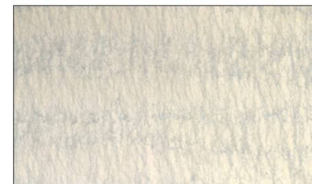
STRAT APLICAT CORECT (20-22 grame / mp)
